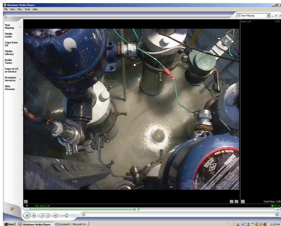
Fig. 1. Appearance of a bubble on the surface of a bumped vessel. The still frame shows a bubble of about 6 cm in diameter emerging from a 0.49 m 3 vessel containing an aqueous slurry of kaolin and bentonite particles. Before the perturbation, the fluid was stationary and contained millions of oxygen bubbles generated by H 2 O 2 decomposition of average diameter 0.3 cm. Bubble coalescence must have occurred to generate the observed bubble since the vessel depth (0.8 m) is too shallow for significant enlargement by decomposition.
