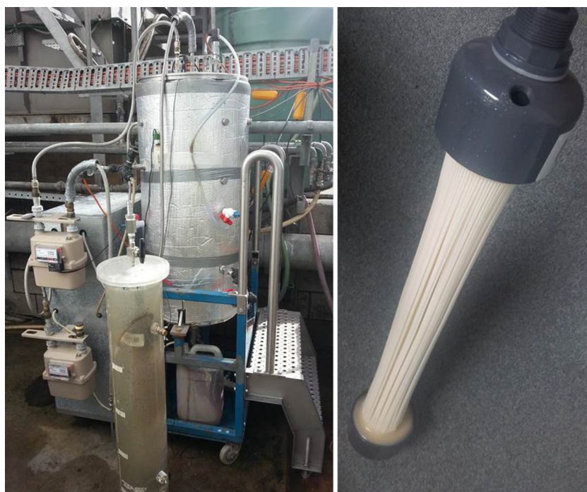
Fig. 1. Anaerobic membrane bioreactor pilot plant installed at an Australia beef processing facility (left) and hollow fiber membrane module (right).
