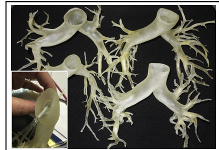
Flexible 3D printed models with inset, showing their use testing a catheter prototype.
