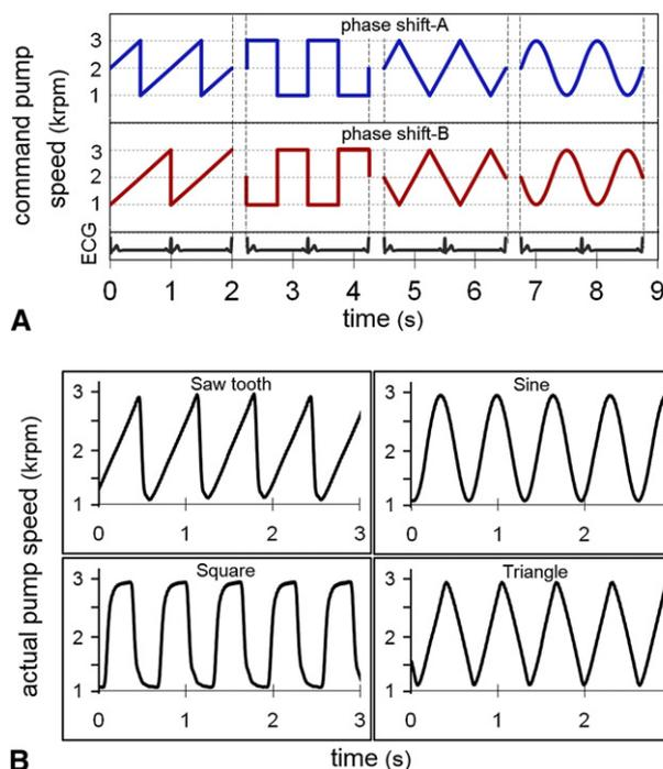
**FIGURE 1.** A, Various types of waveforms synchronized with electrocardiogram (ECG) as pump speed command. Phase shifts A and B have a 180-degree phase difference. krpm is a measure for rotational speed of the pump. B, Actual pump speed derived from the motor's Hall sensors.
