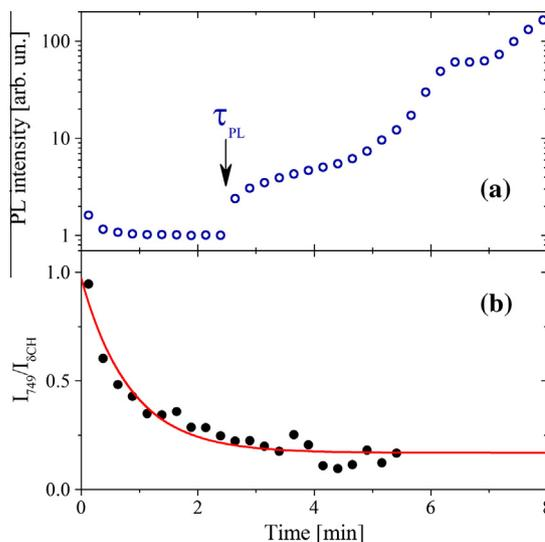
**Fig. 2.** Representative time dependence of the photoluminescence intensity (a) and the  $I_{749}/I_{\delta\text{CH}}$  ratio (b) under 4 mW laser irradiation. The onset of the drastic photoluminescence increase is denoted by the arrow in (a). The exponential decay fit is shown by the solid line in (b).
