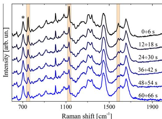
**Fig. 1.** Time-resolved Raman spectra of living yeast cells for 10 mW laser power. The spectra are vertically shifted for convenience. The shadow stripes mark the Raman peaks of cytochrome. The asterisk denotes the contribution from the mica slice.
