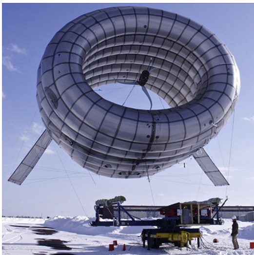
Fig. 1. A prototype of blimp based HAWP generating system developed by Altaeros Energy.
