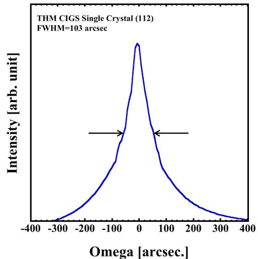
Fig. 2. The XRC of (112) oriented CIGS single crystal.
