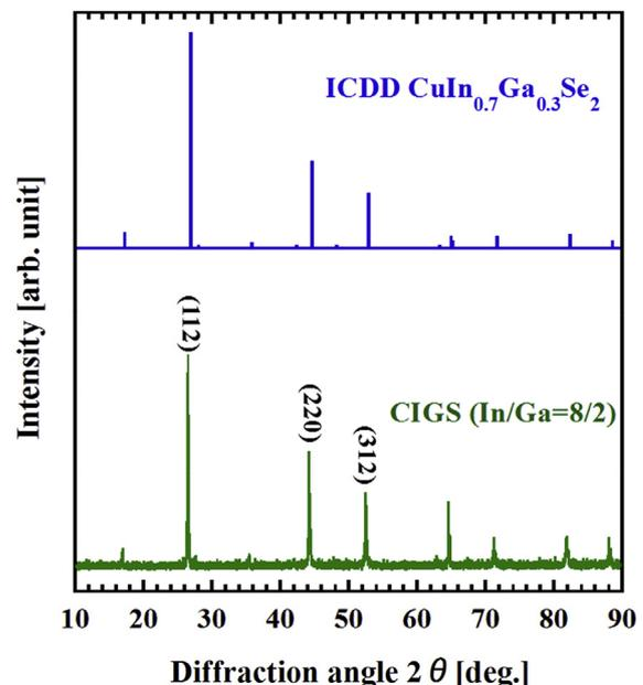
Fig. 3. The powder XRD of the CIGS single crystal grown with  $X = 80\text{ mol}\%$ .
