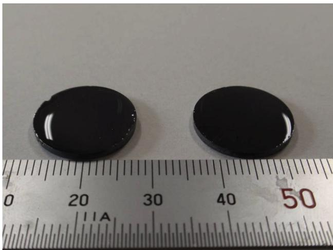
Fig. 1. The photograph of CIGS single crystal wafer.
