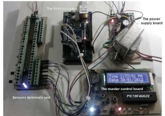
Fig. 1. Photograph of the proposed data acquisition system.
