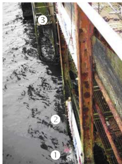
Fig. 1. Corrosion zones on offshore wind power structures investigated in this study (left) and outdoor test stand at Helgoland with specimens and corrosion zones (right) (Photographs: Offshore Wind Net; IFAM, Bremen). 1 – Underwater zone (UZ); 2 – Intermediate zone (IZ); 3 – Splash zone (SZ).
