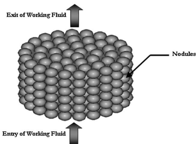
Fig. 1. Arrangement of spherical capsules in LHES system.
