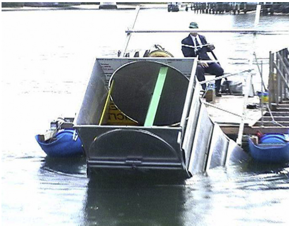
Fig. 1. 1.2 \times 1.2 m turbine in duct, raised to show turbine.
