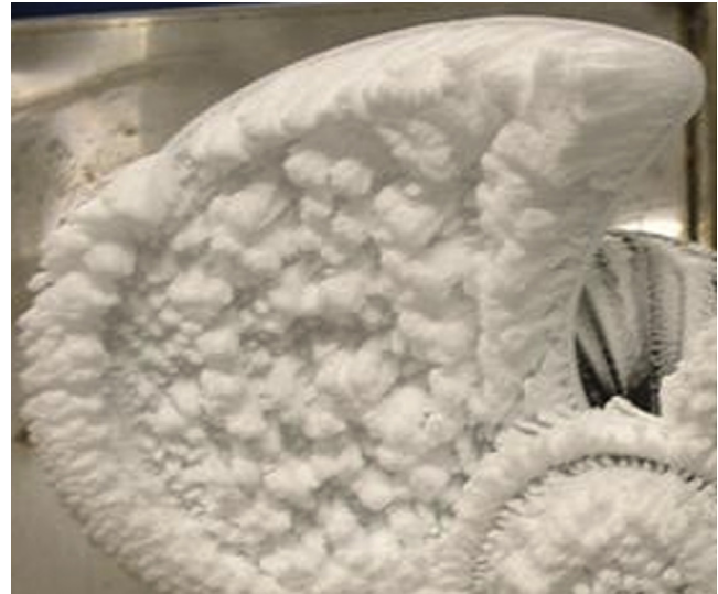
Fig. 2. Rime ice with feathered texture formed on a rotating fan blade.
