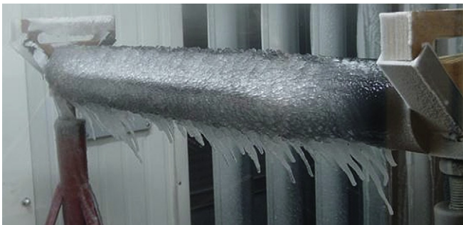
Fig. 1. Glaze ice with frozen rivulets formed in the icing tunnel.
