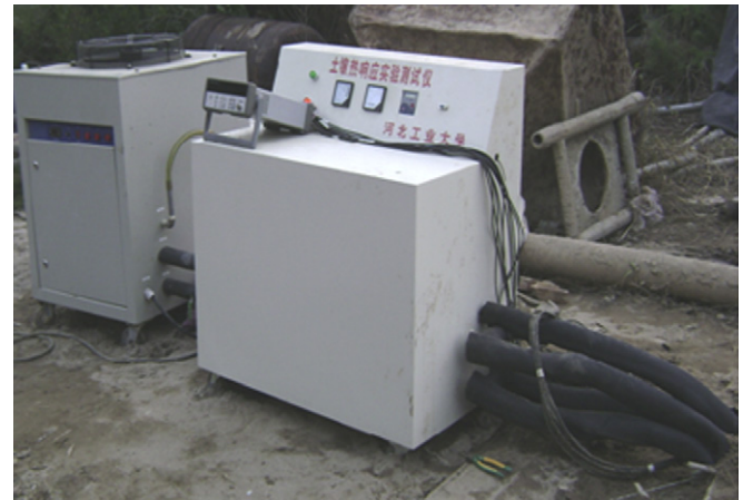
Fig. 2. In situ test photo of the improved TRT equipment.
