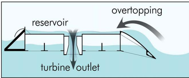
Fig. 1. Overtopping principle.
