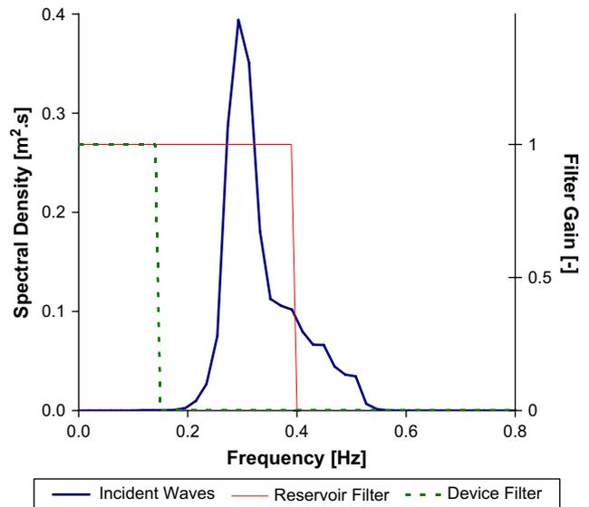
Fig. 4. Frequency spectrum of incident waves for Record 3, and transducer low pass filter gains.
