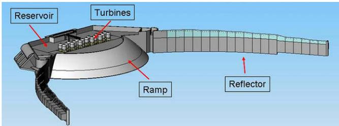
Fig. 2. Layout of the Wave Dragon device.
