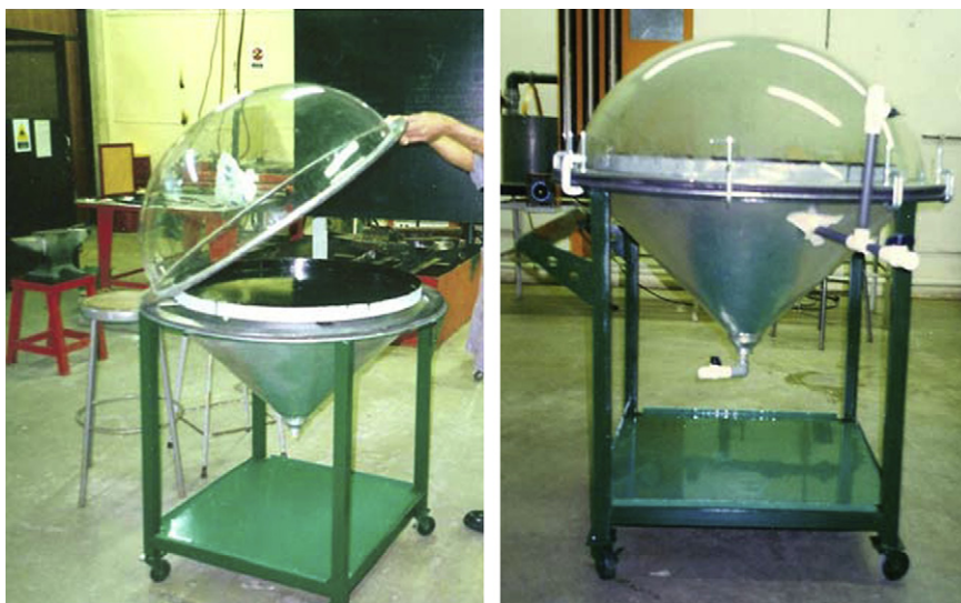
Fig. 2. Photographs of the fabricated hemispherical solar still.
