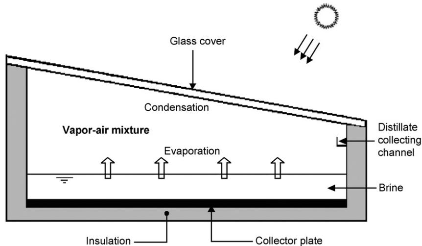
Fig. 1. Schematic view of a solar still.
