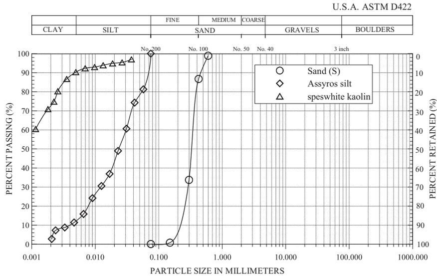
**Fig. 1.** Grain size distributions of sand (S), Assyros silt, and speswhite kaolin, used in the tests.
