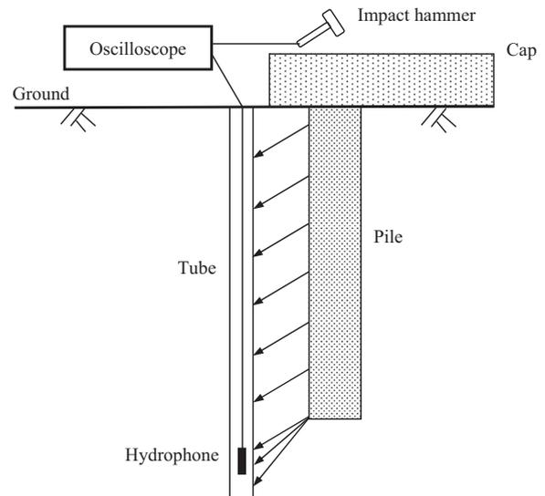
Fig. 2. Specification for integrity by PS test.
