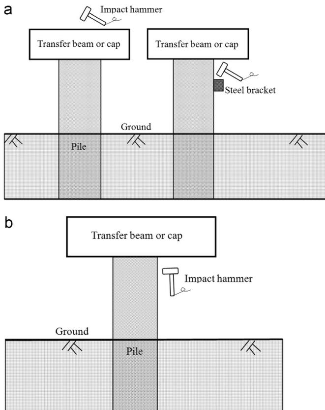
Fig. 1. Schematic arrangement for (a) longitudinal and (b) flexural wave testing.
