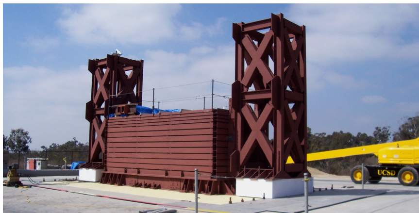
Fig. 3. Restrained laminar soil container on outdoor shake table at UCSD.
