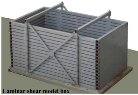
Fig. 1. Laminar shear soil box used in the shaking table model tests.
