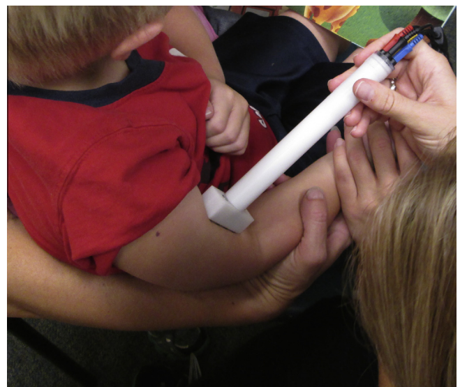
Fig. 1. EIM being performed on the biceps of a young boy with Duchenne muscular dystrophy. The array is placed longitudinally along the muscle. The connectors/wires at the end of the tube attach to the impedance-measuring device (not shown).
