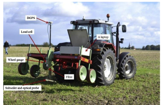
Fig. 1. Multi-sensor platform for the on-line measurement of soil properties (Mouazen et al., 2014).
