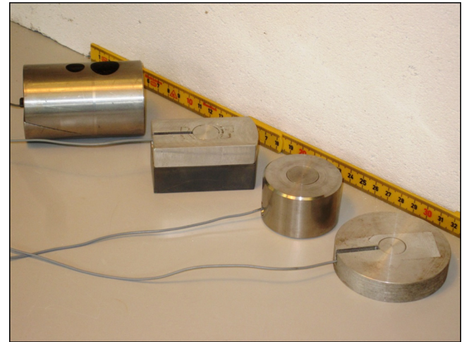
Fig. 1. The four types of transducers used in the study. From left to right: profile DK (load cell under the largest piston); Profile S; Surface DK; Surface S. See Table 1 for transducer dimensions.
