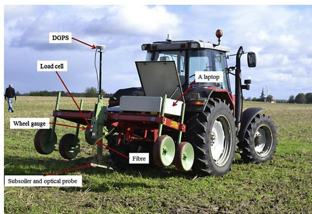
Fig. 1. On-line visible and near infrared (vis-NIR) soil sensor (Mouazen, 2006).
