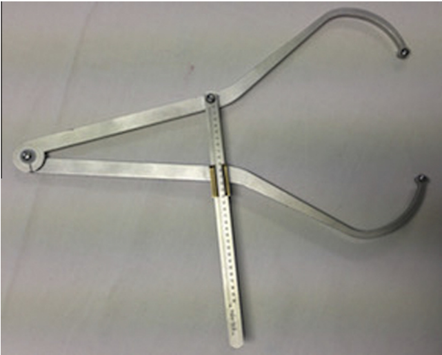
Fig. 1. Metal sliding callipers used to measure the deformity. This figure is available in colour at http://www.sciencedirect.com/ .
