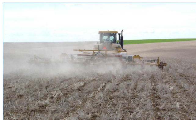
Fig. 2. The undercutter's narrow-pitched and overlapping 80-cm-wide V blades slice beneath the soil at a depth of 13 cm to completely sever capillary channels and halt the upward movement of liquid water to retain seed-zone water in summer fallow for late-summer planting of winter wheat. Most of the winter wheat residue from the previous crop is retained on the surface to control wind erosion. Photo by W.F. Schillinger.
