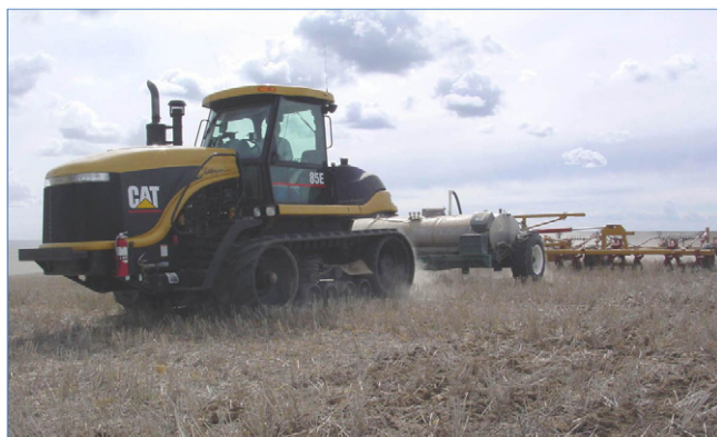
Fig. 1. A 375 horse power crawler tractor pulls a 3800 L tank cart filled with aqua \text{NH}_3\text{-N} and a 10-m-wide undercutter implement during primary spring tillage plus N fertilizer injection during the month of April. Photo by W.F. Schillinger.
