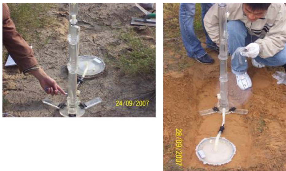
Fig. 2. Pictures of an infiltration experiment on crusted soil and on crust-removed soil.
