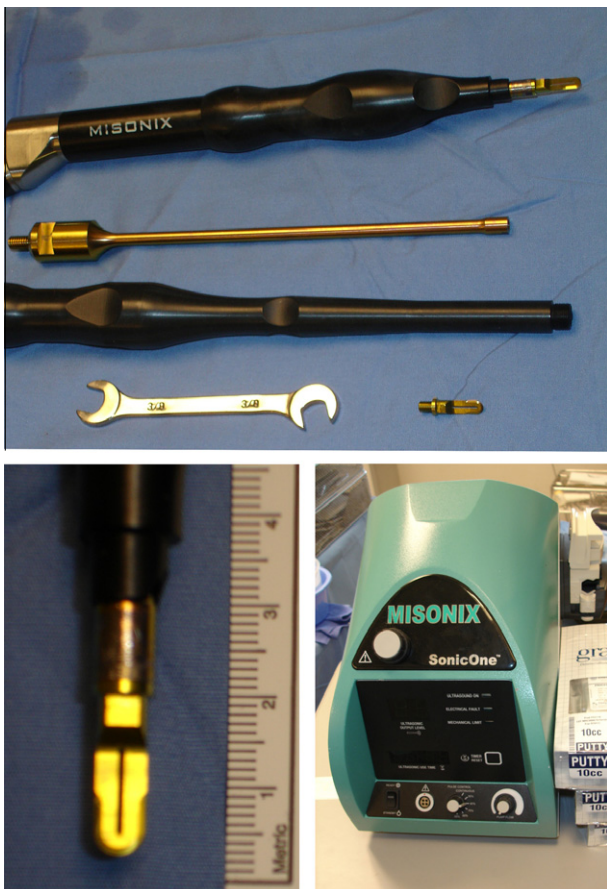
Fig. 1. Photograph showing the Misonix generator and handpiece with attached tip.
