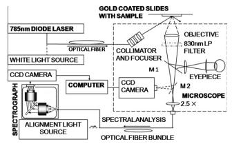
Fig. 1. Setup of the home-made microspectroscopy system.
