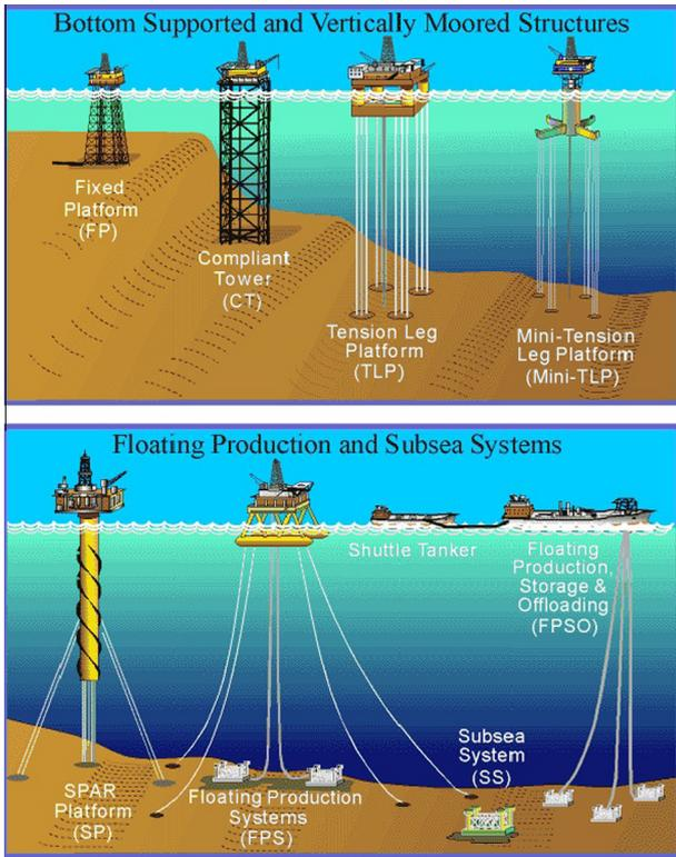
Fig. 1. Schematic of typical energy production facilities in deep water (MMS 2011).
