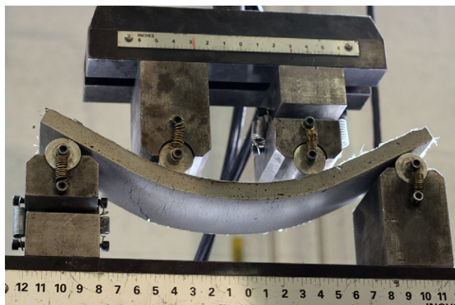
Fig. 1. Fiber reinforcement of cementitious systems can produce distributed micro-cracking and ultra-ductile behavior, leading to increased durability. (Image courtesy University of Michigan News Media).
