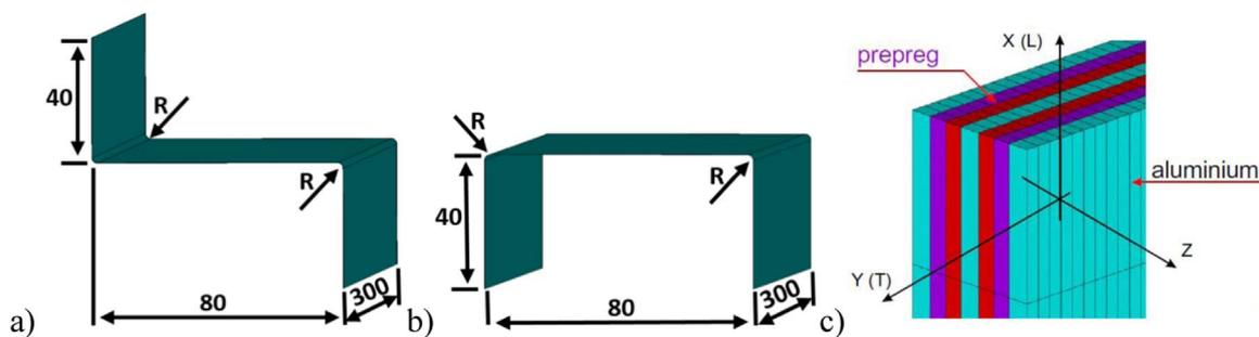
Fig. 1. Overall dimensions of Z-shape (a) and channel section (b) with specific lay-up configuration (c).
