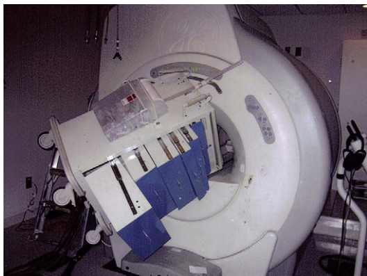
Fig. 2. This photograph taken in a diagnostic MR suite illustrates the risk of violating the spatial magnetic field with an anesthesia cart.
