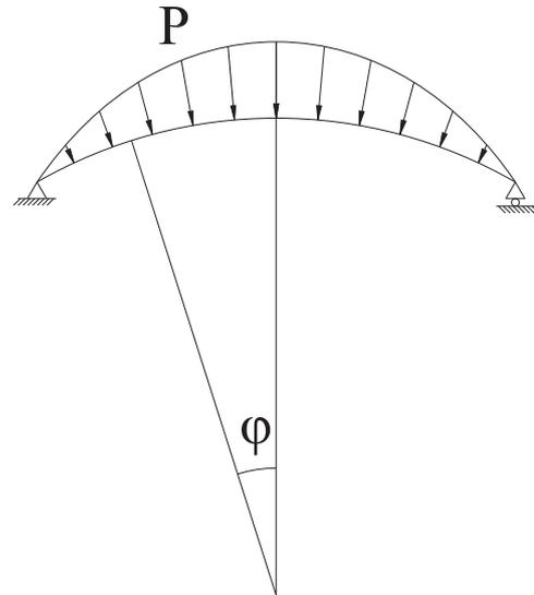
**Fig. 1.** Schematic diagram of the simplified mechanical model in SH3046.
