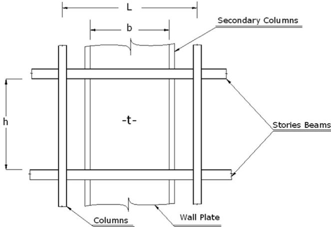
Fig. 1. General shape of semi-supported steel shear wall.
