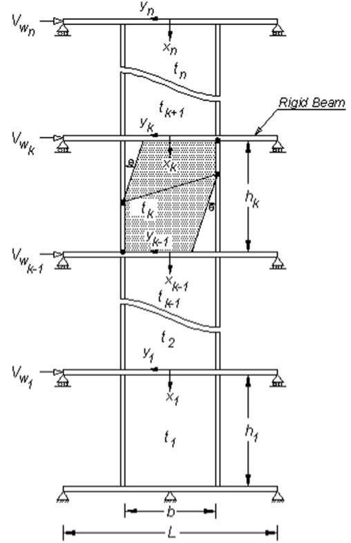
Fig. 2. A semi-supported steel shear wall with rigid beams under lateral forces.
