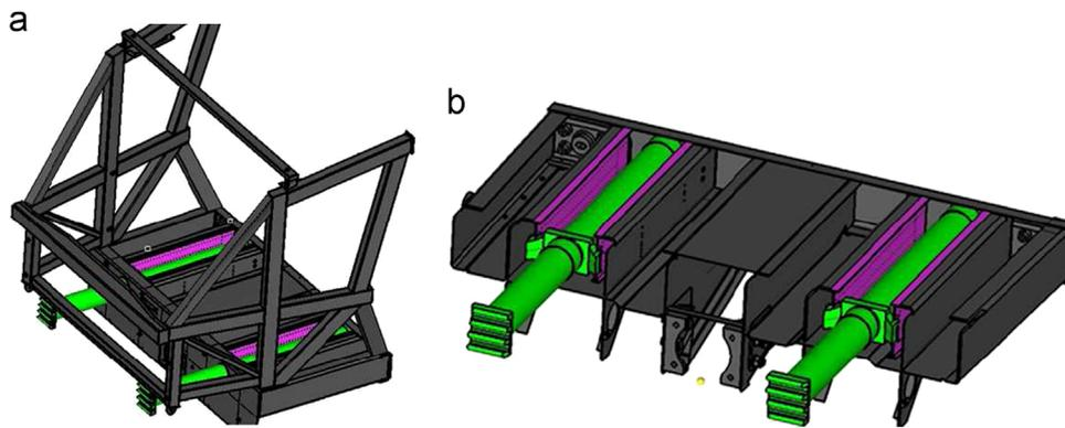
Fig. 1. (a) Absorber mounted in the front part of the wagon structure; (b) enlarged view of the absorber.
