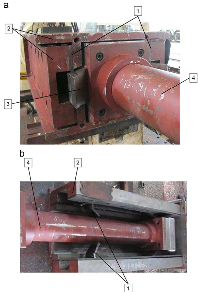
Fig. 2. (a) The appearance of the energy-absorption device; (b) internal view of the structure: (1 – steel plates; 2 – support tool; 3 – die; 4 – guide bar).
