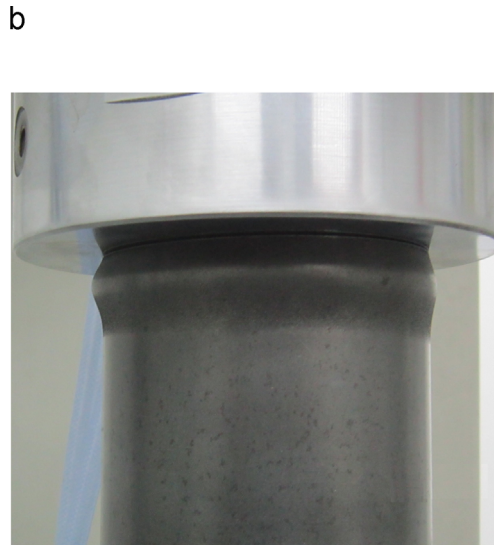
Fig. 1. Geometry of analyzed cylinder (a), a close look of the top edge after spring-back/unloading during experimentation (b).
