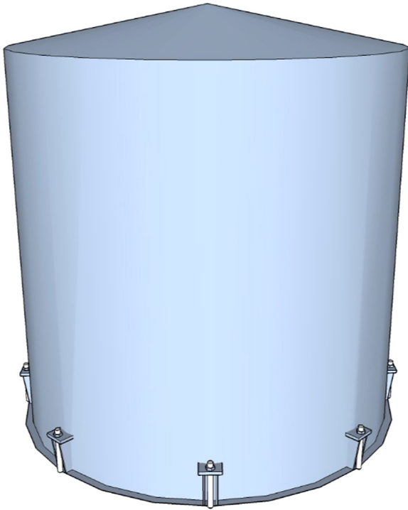
Fig. 1. Typical storage tank with anchor bolt chairs.
