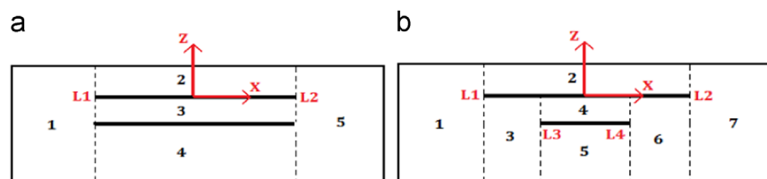
Fig. 1. Division of the laminate with multiple through-the-width delaminations into regions. (a) Equal length delaminations (b) Delaminations with different lengths.
