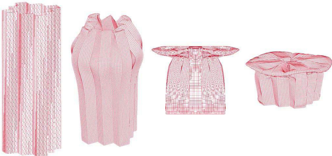
Fig. 1. The non-compact expansion-contraction deformation mode of non-convex thin-walled column.
