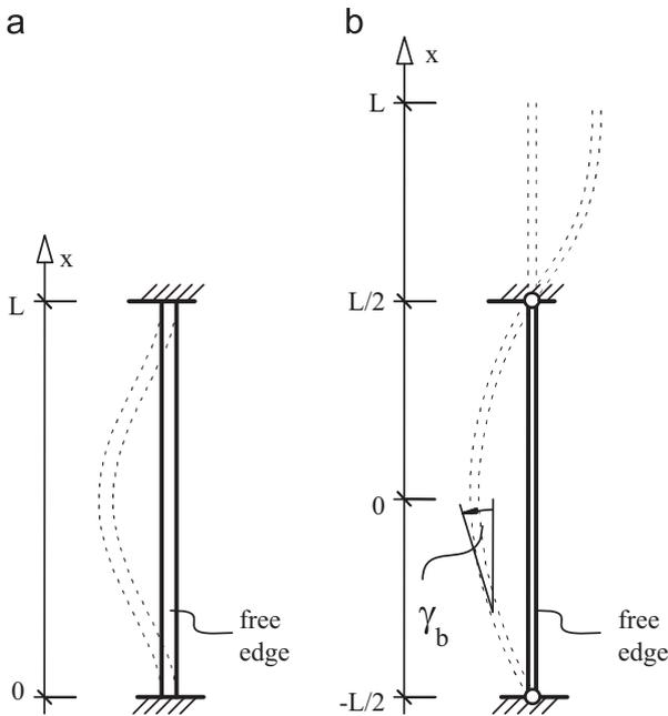
Fig. 1. Fixed and pinned end conditions. (a) Fixed-ended boundary conditions, (b) Pin-ended boundary conditions.
