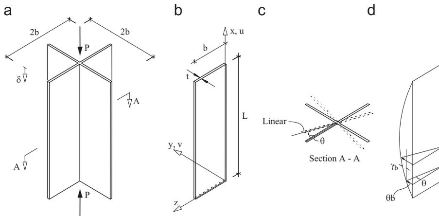
Fig. 2. (a) Cruciform in compression, (b) flange element, (c) torsional buckling, and (d) fibre rotation.
