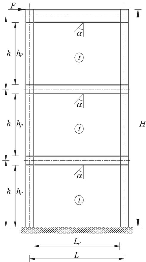
Fig. 1. Geometric configuration of three-story single bay SPSW.
