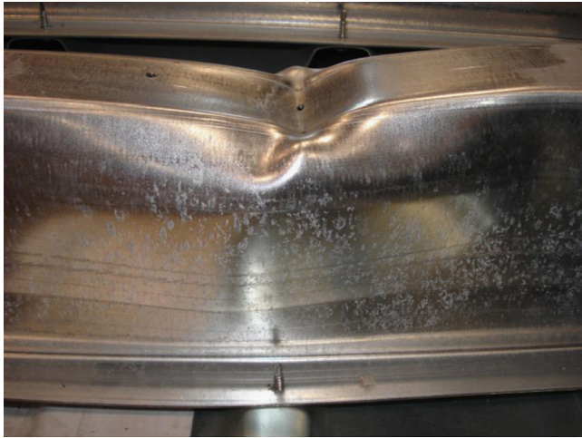
Fig. 1. Flange crushing in a hat-section beam acted by a concentrated load.
