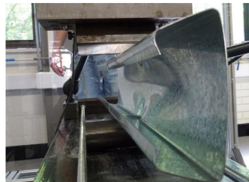
Fig. 2. Web crippling failure at a support [2].
