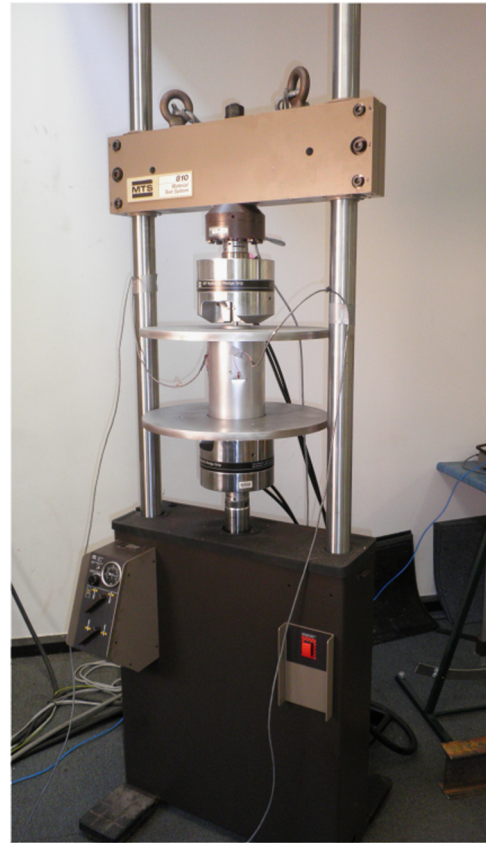
Fig. 1. Test set-up for cylindrical shell specimens.
