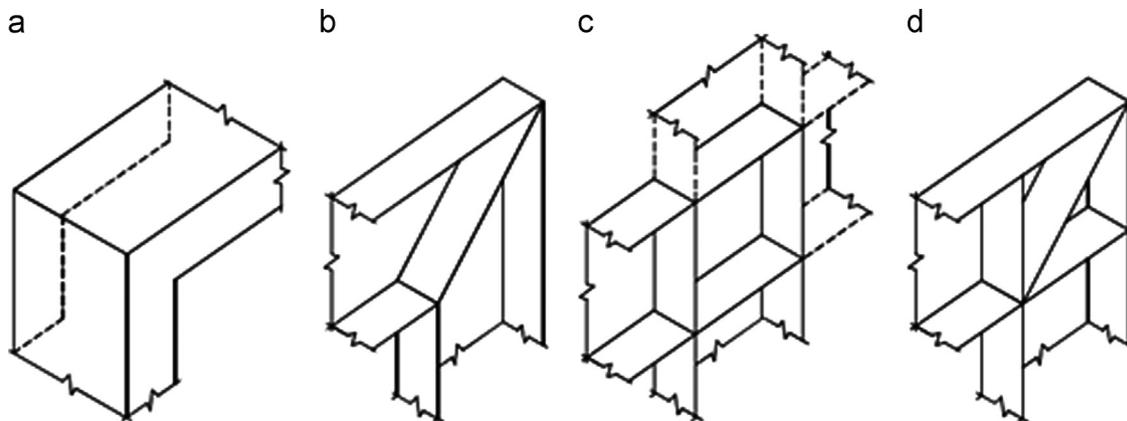
Fig. 1. Configurations of joints between channel members [28]: (a) unstiffened with flange continuity, (b) diagonal stiffened, (c) box stiffened, (d) diagonal/box stiffened joints.
