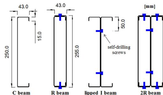
Fig. 1. Scheme of the cross-sections of the tested beams.
