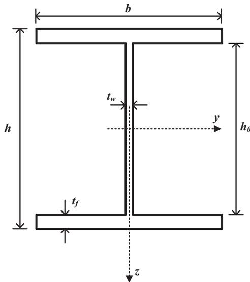
Fig. 1. Simplified cross section of an I-shaped steel member.
