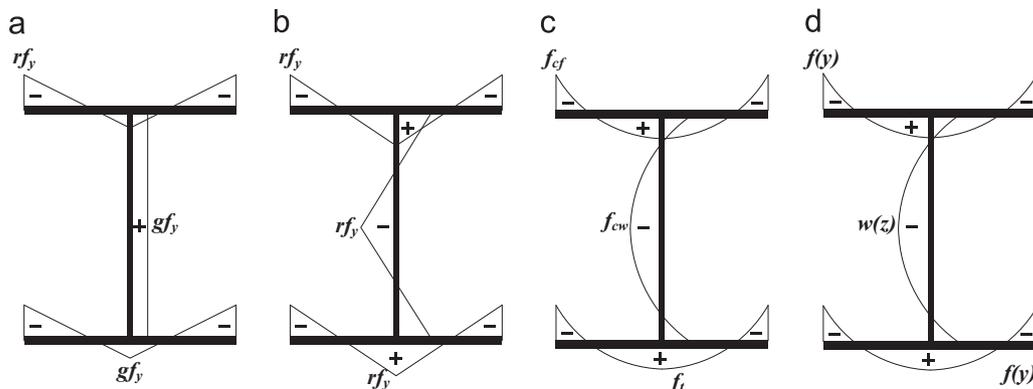
Fig. 2. General residual stress distributions: (A) linear (Galambos and Ketter [9]), (B) linear (ECCS [10]) (C) parabolic (Young [12]), and (D) parabolic (Szalai and Papp [11]).
