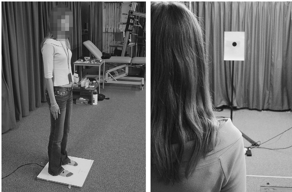
Fig. 1. Balance test using an electronic platform. Subjects are instructed to stand right up (see panel left) for 1 min with eyes closed and 1 min with eyes open, focusing on a target point (see right panel). Reprinted with permission from QinetiQ.
