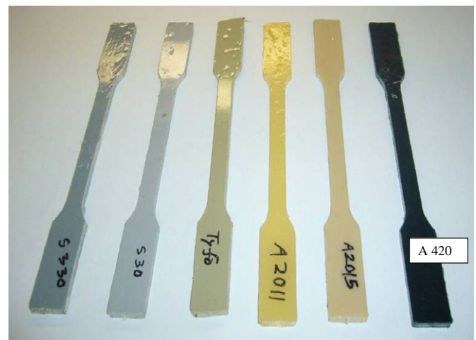
Fig. 1. Six different adhesives tensile coupon test specimens.
